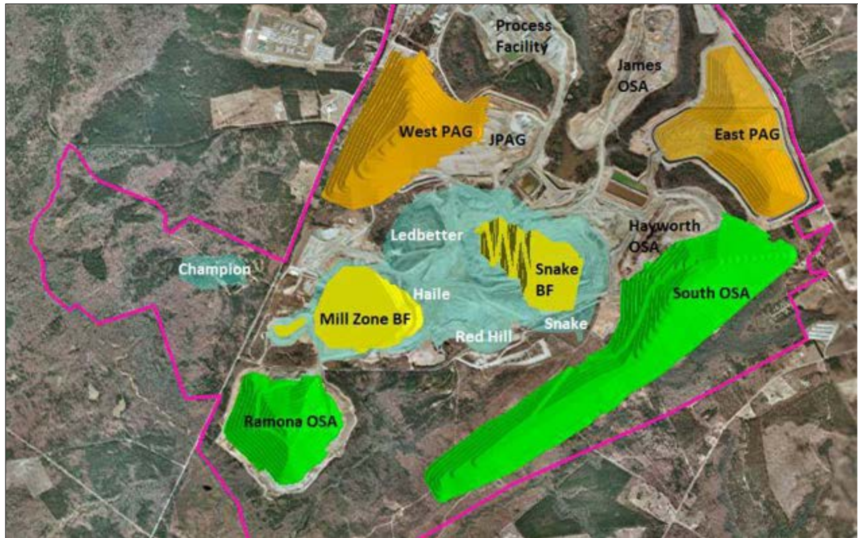
Figure 16-7: Final Pit Design and Ultimate Overburden Storage Site Plan
