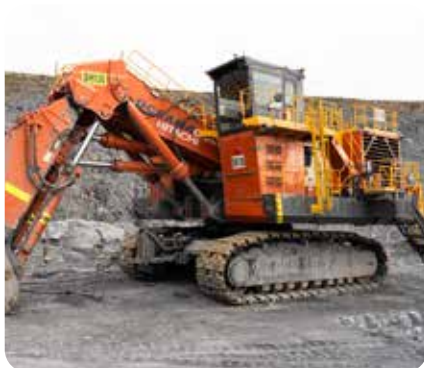
A Hitachi EX3600 electric hydraulic shovel used at our Macraes Operation, New Zealand
