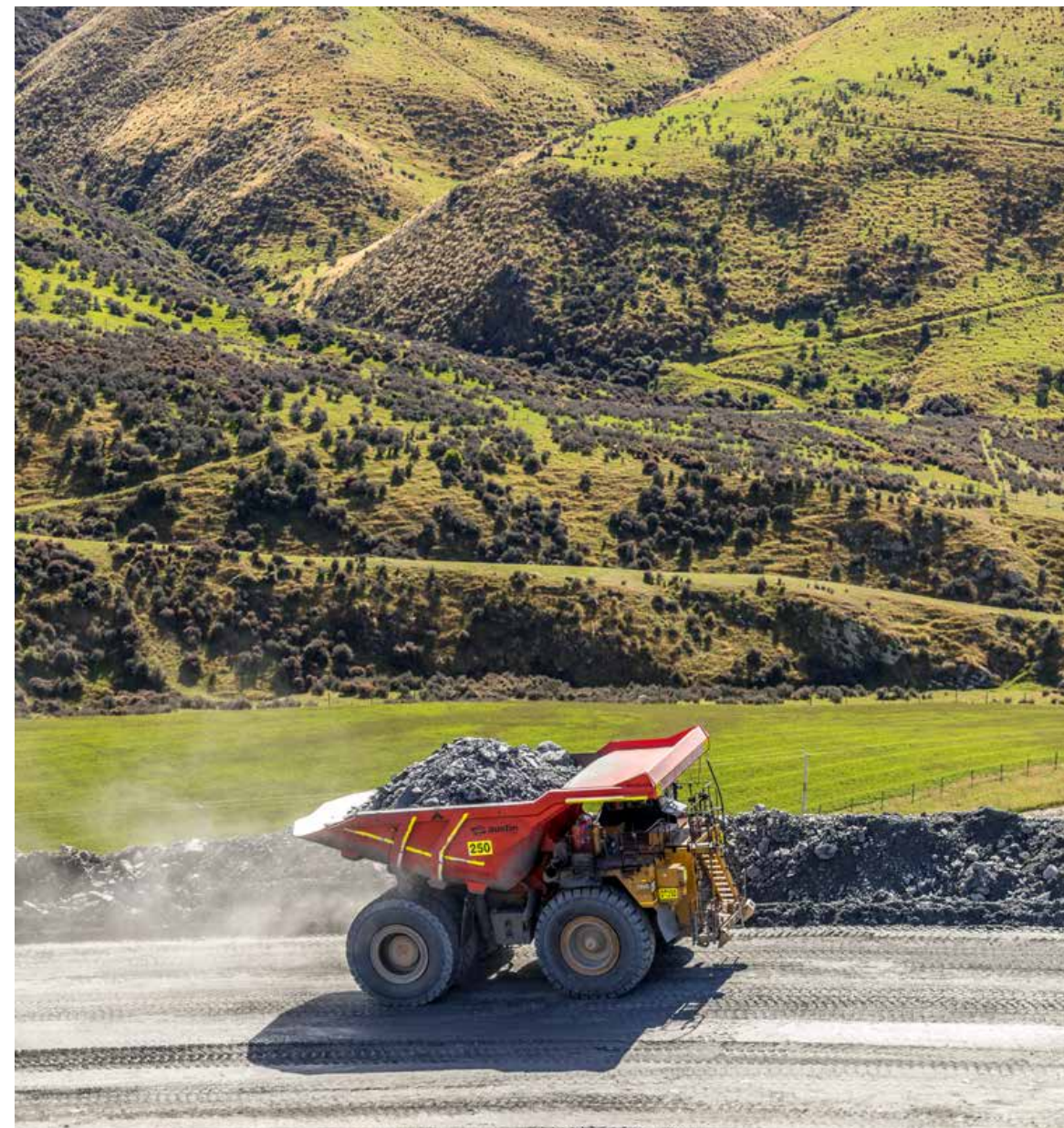
Haul truck at our Macraes Operation, New Zealand. The truck's tray is new and lightweight, which increases haulage capacity and can assist in reducing diesel use and associated emissions.
